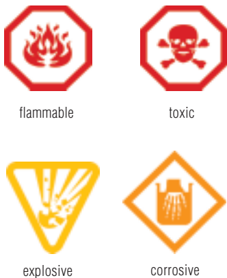
FIGURE A1.2 Hazard symbols indicate both the type of hazard and the degree of hazard.
