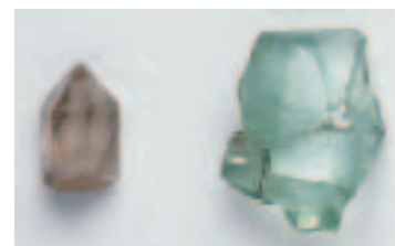
FIGURE A1.7 The formation of crystals is a physical property that can be used to classify substances. On the left is a typical crystal formed by the mineral quartz ( \text{SiO}_{2(s)} ). Glass (right) is an amorphous substance: it never forms crystals.
